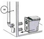
Reconnect the Toilet to the flue pipes and power source.
