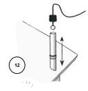
Carefully drop the cleaning set into the vertical vent pipe. Pull the broom slowly up and down the flue pipe to remove ash and debris.
